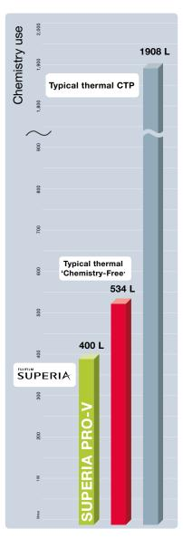
This graphic highlights the amount of chemistry used by different plate solutions. The calculations assume 10,000 B1 plates are produced over a 1-3 month period.
